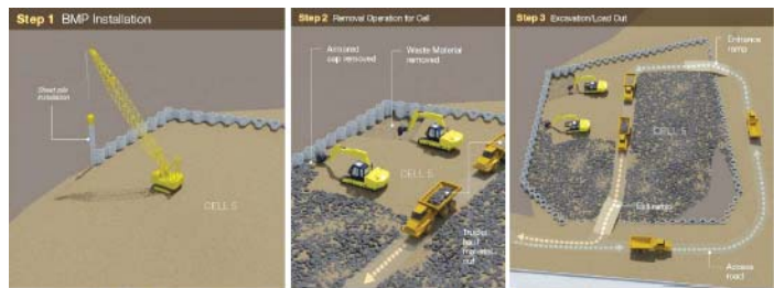
Removal method of dry waste inside cofferdam
