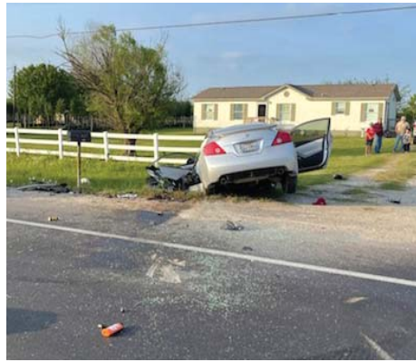
This automobile ravelled fartherest past the point of impact across the highway and into a ditch. the left front of the vehicle is crushed in completely. This car seems to have been eastbound.
