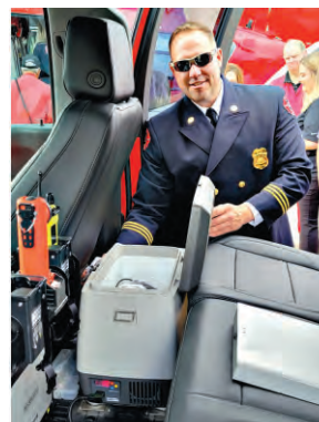
Steve Adams, CFD Assist. Chief of EMS shows the on-board refrigeration unit on their Blood Mobile. The blood is fresh low titer O+ whole blood. The temperature must be maintained at all times to 2-6 C (35.6 - 42.8 F). The vehicle has a blood warmer that raises the blood temperature to 38 C (100.4 F) in ten seconds before it's given to a patient. (Photo by Allan Jamail)
