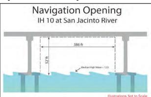
The new roadway will be 30' higher than existing. The navigational opening for boats is increased in height and width to reduce impacts to the bridge structure and bumpers.
