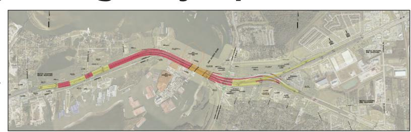
New Highway and Bridge construction stretches for 4.5 miles, from Magnolia Street to Thompson Road. New ramps will connect Spur 330 to I-10. In this schematic, Orange denotes steel bridges, Red concrete, and Yellow on-grade construction. All work is within the existing right-of-way plus 5.4 acres additional. These red lanes will be 30' above existing roadbed.
